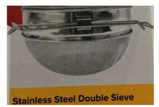
For those of you familiar with the stainless-steel double sieves commonly used to filter honey, the top filter measures in 20 meshes (841 microns) and the bottom fine filter measures in 40 meshes (420 microns). That is plenty adequate for hobby beekeepers. Filters are available for 5-gallon buckets in the range of 600 micron to 200 micron at very reasonable cost.
