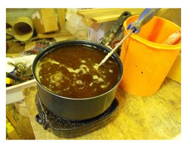
First, wax must be melted and remain heated in a liquid state. A temperature above 148 degrees F. is required. One must not let the wax reach a boiling point. Avoid burns caused by hot wax. Arm coverings are important as well as the possibility that if tipped or spilled, hot wax can cause serious burn injuries. More than one house has burned to the ground by someone melting bees wax on the kitchen stove.
